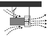
During unit operation, water is circulated from 360° around the unit. The Circulator draws in water and circulates it throughout the pond.
