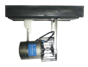
The motor unit attaches to the float using stainless steel hardware for an easy and secure assembly. The single piece, rectangular, U.V. resistant, high density thermoplastic float allows for excellent durability with low visibility. The 5 position angling plate allows for multiple angle settings with a simple adjustment.
